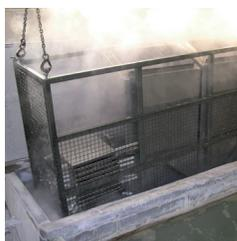
Prior to the application of paint, one of the best processes to begin with is chemical pre-treatment. This entails submerging the product in three different chemical baths to clean, degrease and apply a conversion layer.
